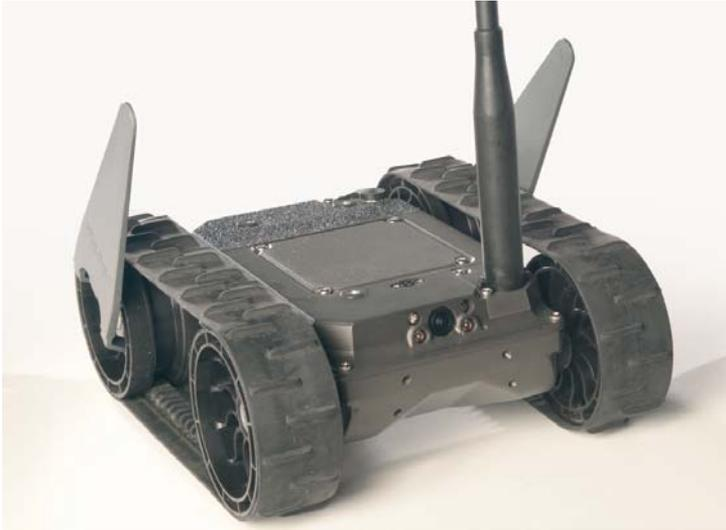
**Figure 1.3:** An example of a small military robot, suitable for use as a LANdroid. It uses tracks for locomotion and has two powered paddles for passing obstacles or righting itself if it lands upside down. (Copyright: iRobot Corp.)
