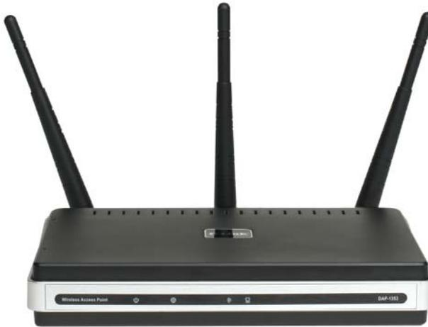
**Figure 2.5:** A wireless access point using spatial diversity to overcome multipath fading. The frequency is 2.4 GHz, so the antennas are spaced about half a wavelength, or 6 cm. (Copyright: D-Link Corp.)
