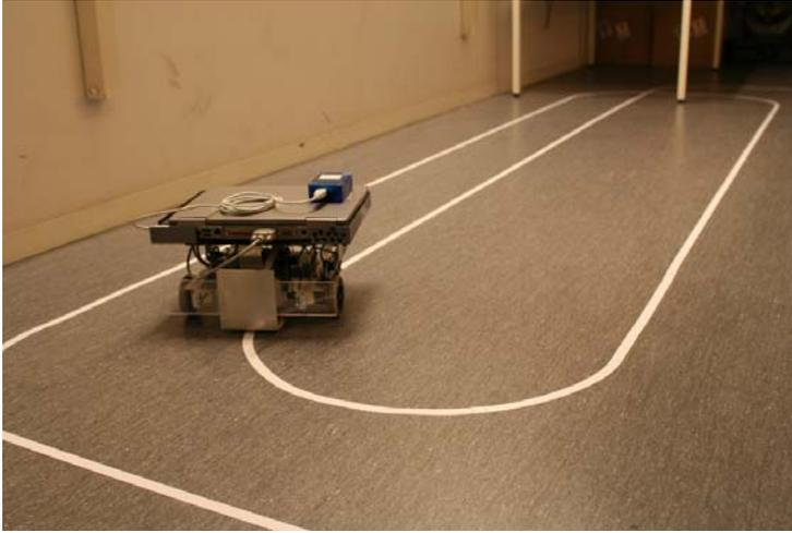
**Figure 4.9:** Experiment setup in the basement lab. The robot follows a tape path on the floor, while the attached Tmote Sky transceiver receives signals from another Tmote Sky in the back of the room.
