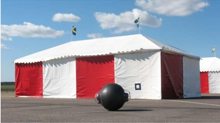
**Figure 1.1:** A GroundBot rolling past a tent at the final demonstration of the AURES project (Ögren et al., 2009). The project demonstrated autonomous capabilities such as positioning for camera surveillance, minimum-time patrolling and searching and securing designated areas.
