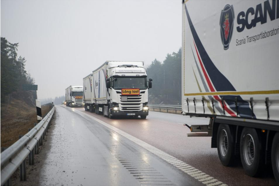
Figure 1.4: Heavy-duty vehicles in a platoon. Source: Scania
