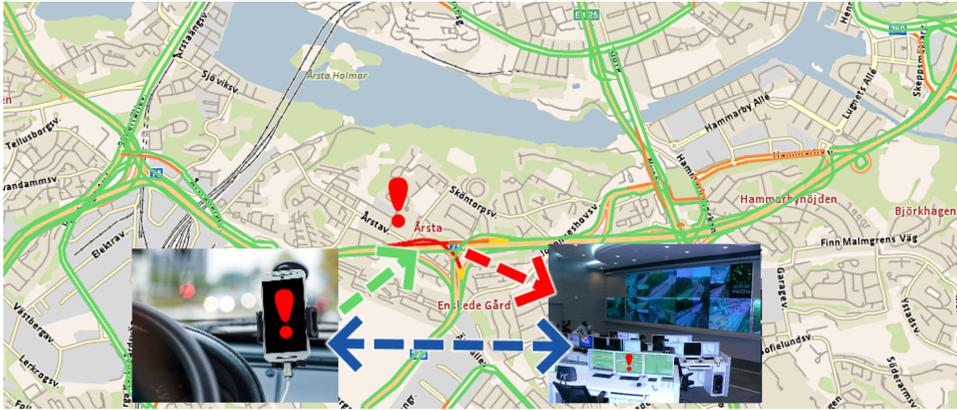
Figure 1.3: A traffic control loop closed via an app. The traffic control centre uses the trajectories of the participating app-connected vehicles, and uses it to estimate the traffic situation. Then the control centre issues reference speed to the drivers through the app. The participating drivers are rewarded monetarily, or with services.
