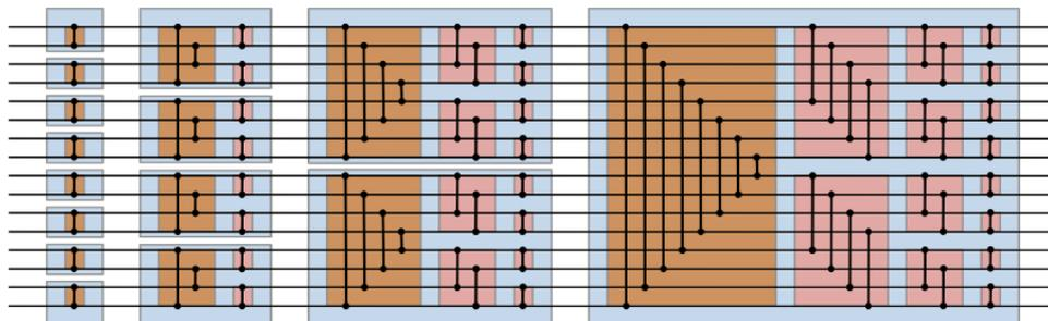
Figure 1: A bitonic sort network of size 16.
