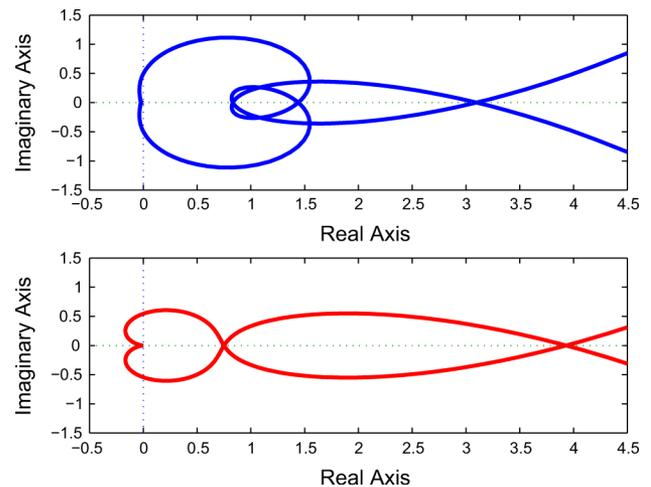
Fig. 8. Nyquist plots of the loop gains  $PC_4$  (above) and  $PC_{opt}$  (below), respectively.
