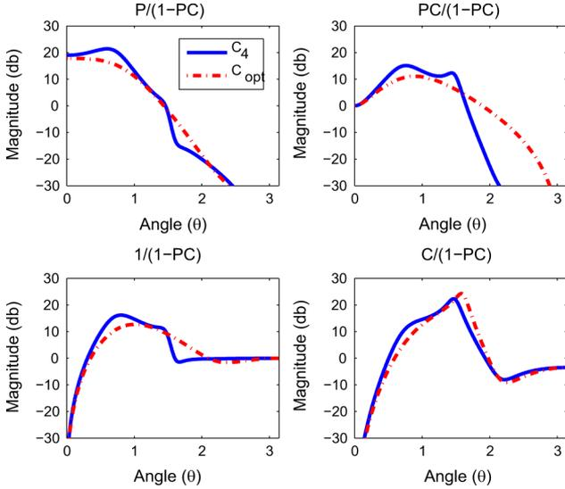
Fig. 9. Four closed-loop transfer functions of  $\Pi_{P/C_4}$  and  $\Pi_{P/C_{opt}}$ .
