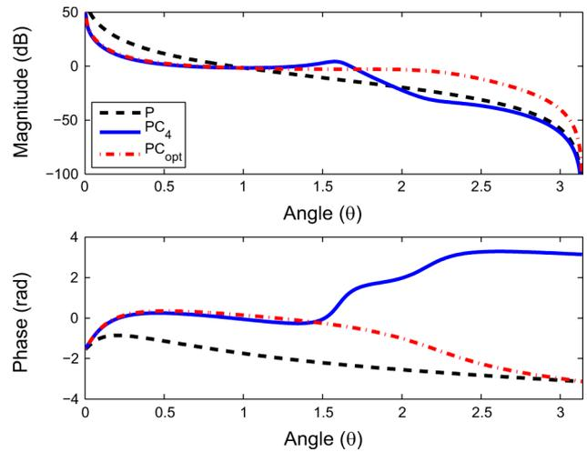
Fig. 7. Bode plots of  $P$  and of loop gains  $PC_4$ , and  $PC_{opt}$ .
