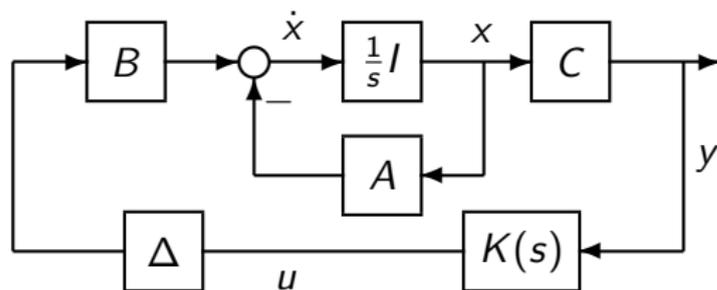
Figure 2: Feedback system with time-varying input delay.
