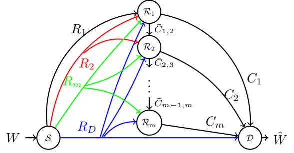
Fig. 2. The upper bounding model from network equivalence theory where the orthogonal channels from relays to the destination are replaced by bit-pipes with rate  $C_i = \max_{P_{X_i}} I(X_i; \tilde{Y}_i)$ , channels from  $\mathcal{R}_i \rightarrow \mathcal{R}_j$  are replaced by bit-pipes with rate  $\tilde{C}_{i,j} = \max_{P_{\tilde{X}_{i,j}}} I(\tilde{X}_{i,j}; \tilde{Y}_{i,j})$ , and the BC from the source is replaced by hyper-arcs with rates  $R_1, R_2, \dots, R_m$  and  $R_D$ .
