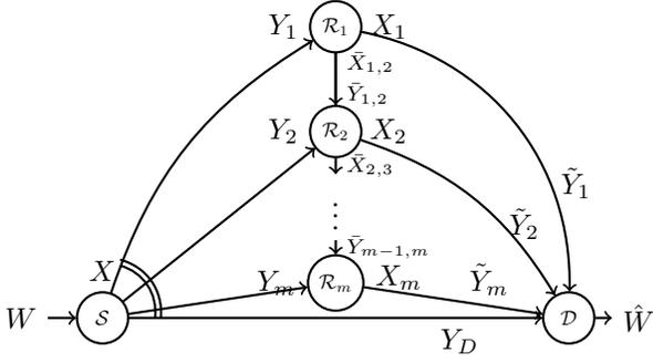
Fig. 1. Wireless relay network where the source  $S$  transmit a message  $W$  to destination node  $D$  via the wideband fading channel with average transmit power constraint  $P$ . This transmitted signal is over heard by  $m$  relay nodes. Channels between relay nodes and from relay to destination are orthogonal.
