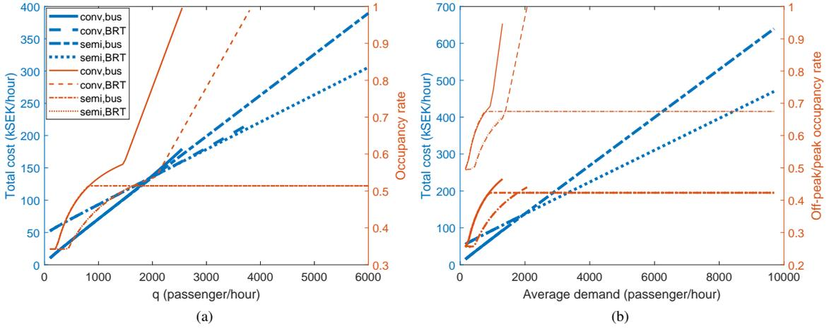
Figure 10: Results of total cost and occupancy rate with respect to (a) demand  $q$  (one-period analysis) and (b) average demand  $\bar{q}$  (two-period analysis). Bus headway is restricted to no less than 3 minutes and BRT headway is restricted to no less than 2 minutes,  $q_2/q_1 = 3$ , other parameters according to Table. 1. (a) and (b) share the line styles, except in (b) the wider occupancy rate lines are for off-peak hours and the thinner for peak hours.
