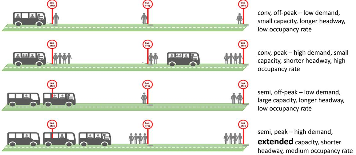
Figure 3: Service operations during off-peak and peak hours with conventional and semi-autonomous vehicles.
