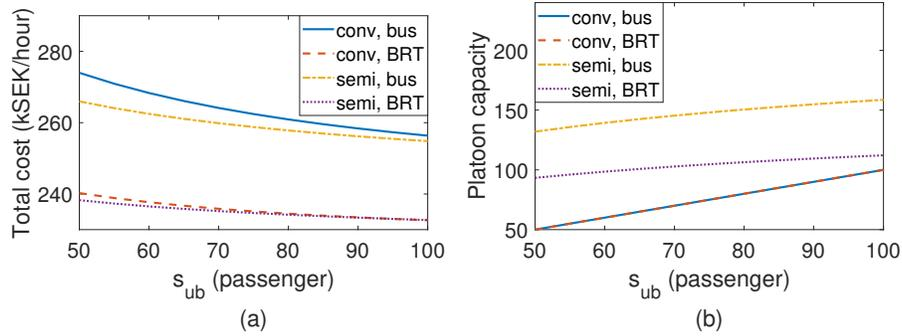
Fig. 2: Results with respect to different upper bound  $s_{ub}$ ,  $q = 4000$  pax/hour.
