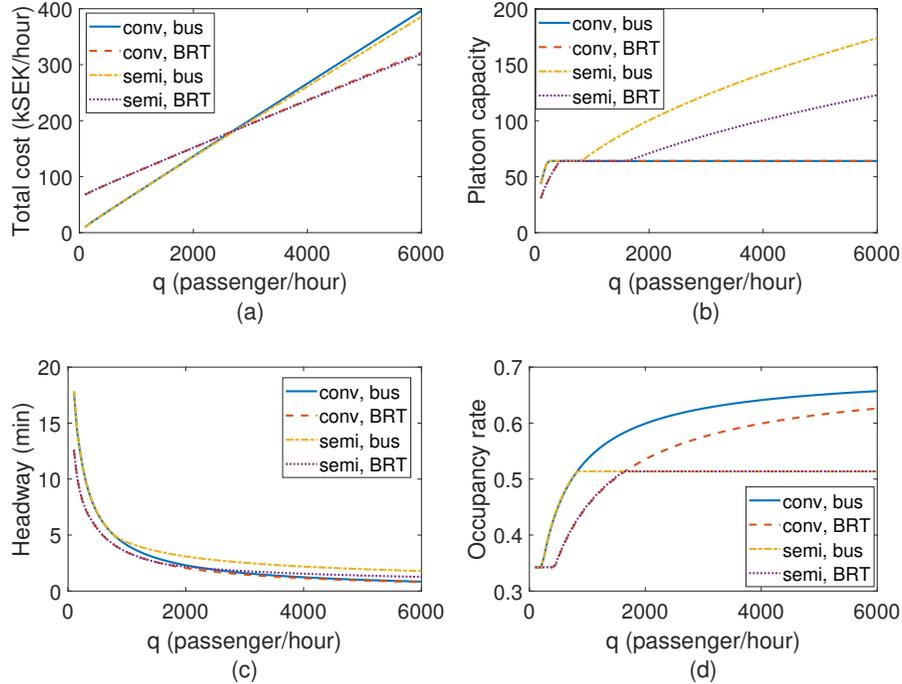
Fig. 1: Results with respect to different demand levels,  $s_{ub} = 64$  pax.
