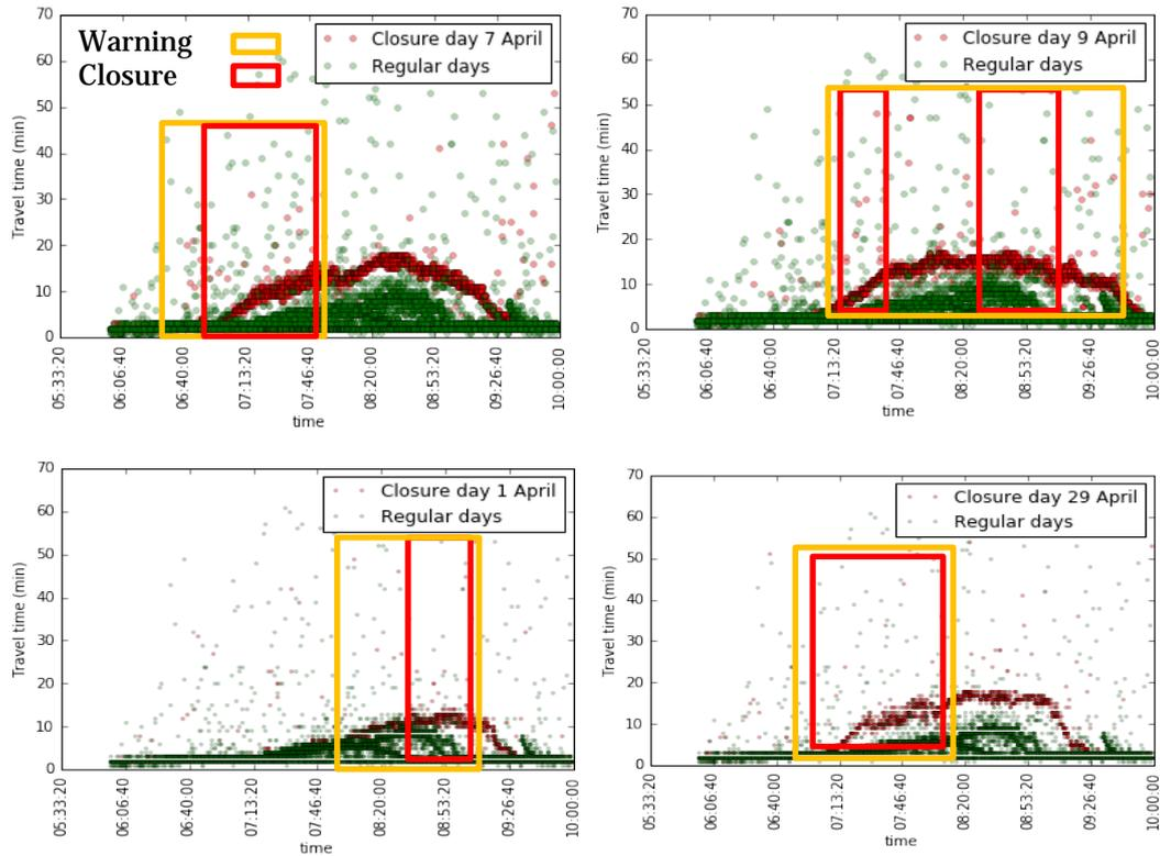
**Fig. 11** Travel time for regular and closure days for the ANPR route.
