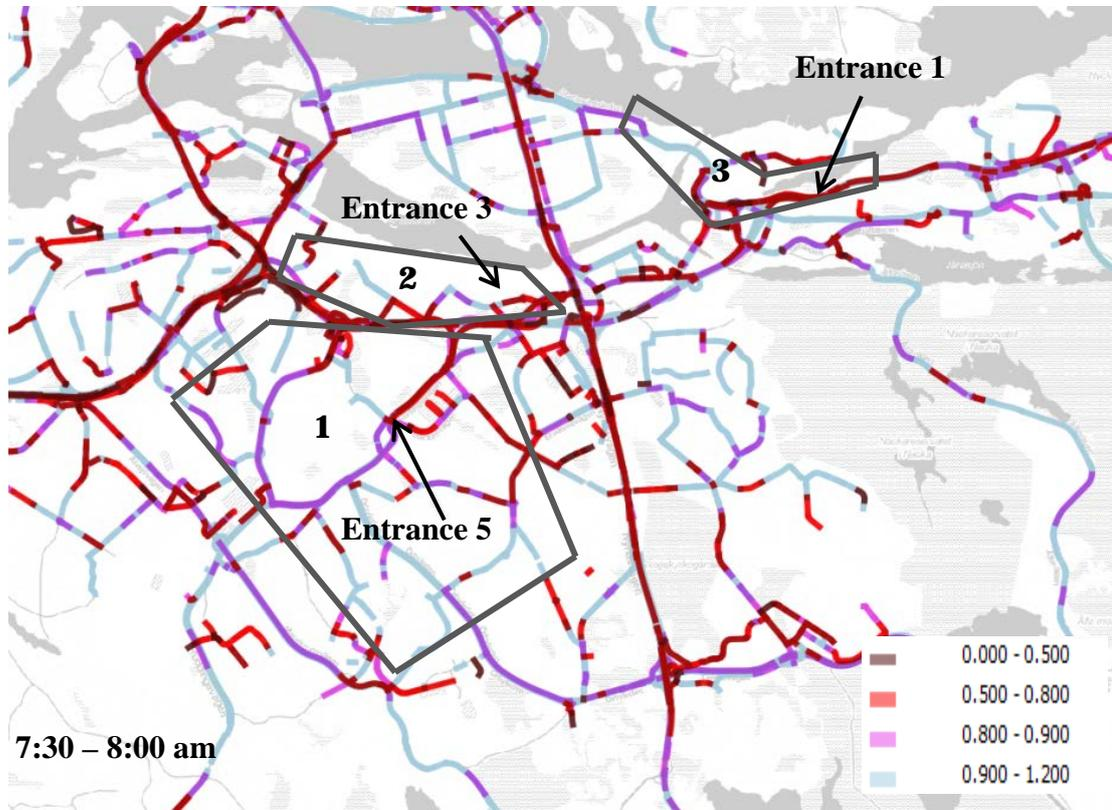
**Fig. 9** Average link speed ratios (closure to regular days, 7:30–8:00 am).
