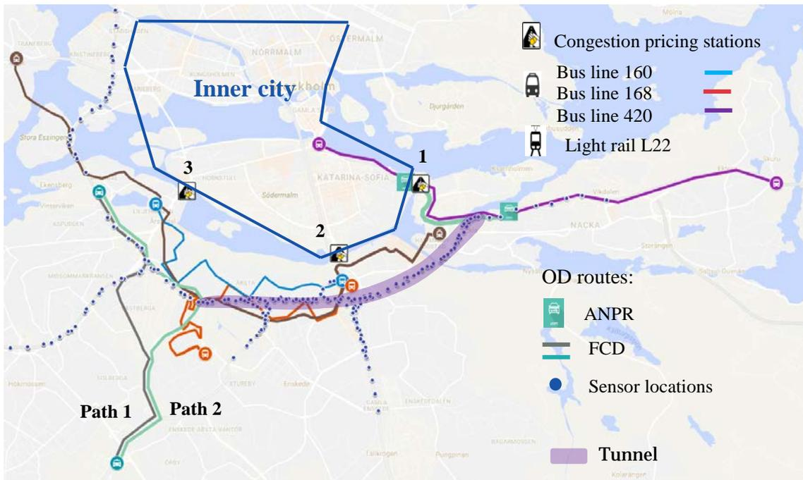
**Fig. 6** Location and coverage of data sources.
