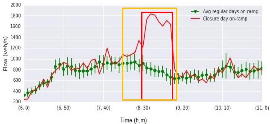
**Fig. 7** Comparison of flow at entrance 2 of a closure day (April 1<sup>st</sup>) and regular days.
