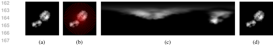
Figure 1: (a) A simulated 64 \times 64 projection image of PDB ID 2pkq. (b) The projection image with a polar grid superimposed (downsampled by a factor of four for visualization purposes). (c) The polar representation. The horizontal axis represents angles and the vertical axis represents radii. (d) The reconstructed image with relative mean squared error 3.5 \cdot 10^{-4} .
