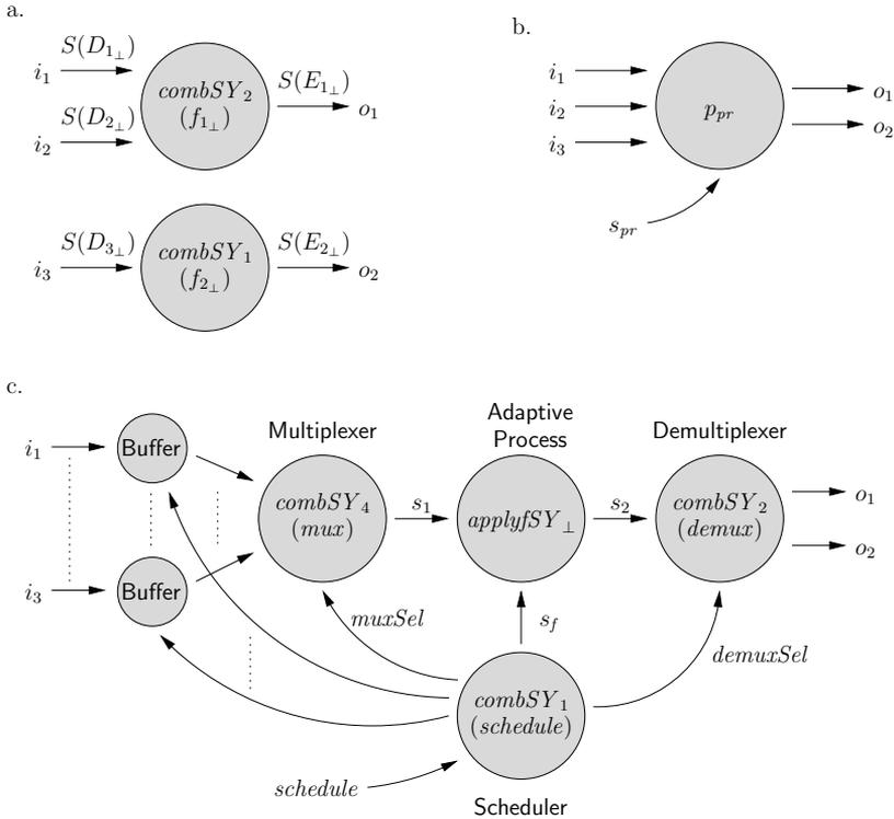
Fig. 13. Figure 13 illustrates the use of an interfaces adaptive process for resource sharing. The processes  $combSY_2(f_{1\perp})$  and  $combSY_1(f_{2\perp})$  shall use the adaptive process as shared resource (Figure 13a). Figure 13b shows an interface adaptive process that is configured by a signal carrying processes as signal values. Figure 13c shows a refined model using a function adaptive process, buffer processes, scheduler, multiplexer and demultiplexer processes.
