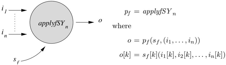
Fig. 9. The process  $applyfSY_n$  models an adaptive process, where adaptivity is controlled by an input signal carrying functions.
