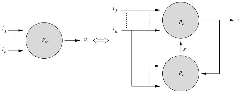
Fig. 8. A self-adaptive process is modelled as a process network of an adaptive process and an additional process. The signal  $s$  can either carry modes, functions or entire processes as illustrated in Figure 7.
