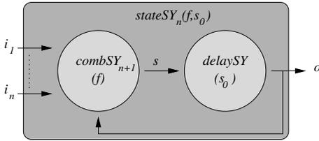
Fig. 6. The process constructor *stateSY<sub>n</sub>* creates a synchronous process that models a state machine without output decoder.
