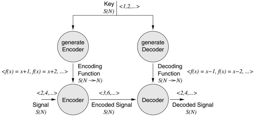
Fig. 11. The Encoder/Decoder is a typical example for function adaptivity. The processes Encoder and Decoder are both function adaptive processes and are fed with signals carrying functions. The types of all signals are shown in the figure.
