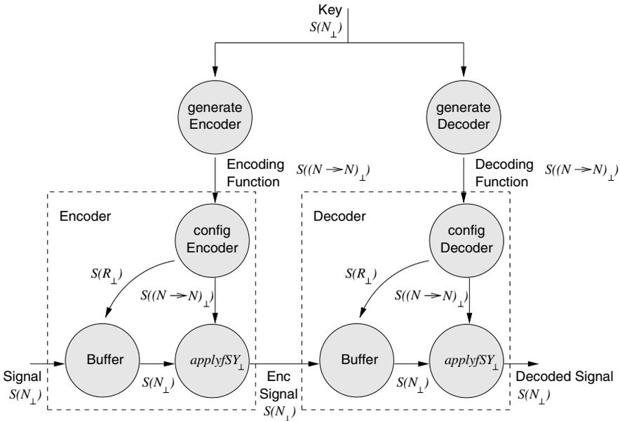
Fig. 12. The refined model of the Encoder/Decoder example takes adaptation time into account. Buffers are introduced and signal types are extended to contain the absent value  $\perp$ . The occurrence of absent events requires the introduction of a buffer that stores the values of the input signal during adaptation. The types of all signals are shown in the figure.
