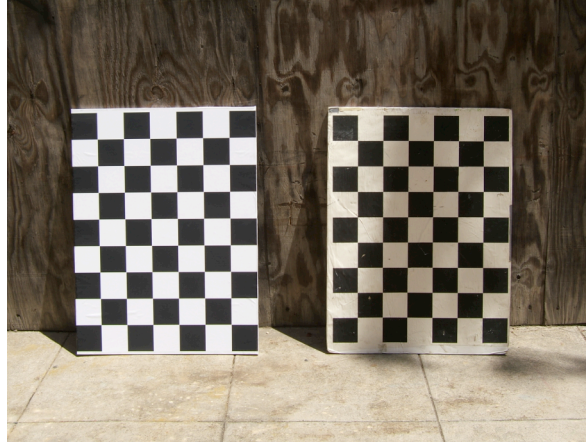
Figure 3: New and old calibration targets
