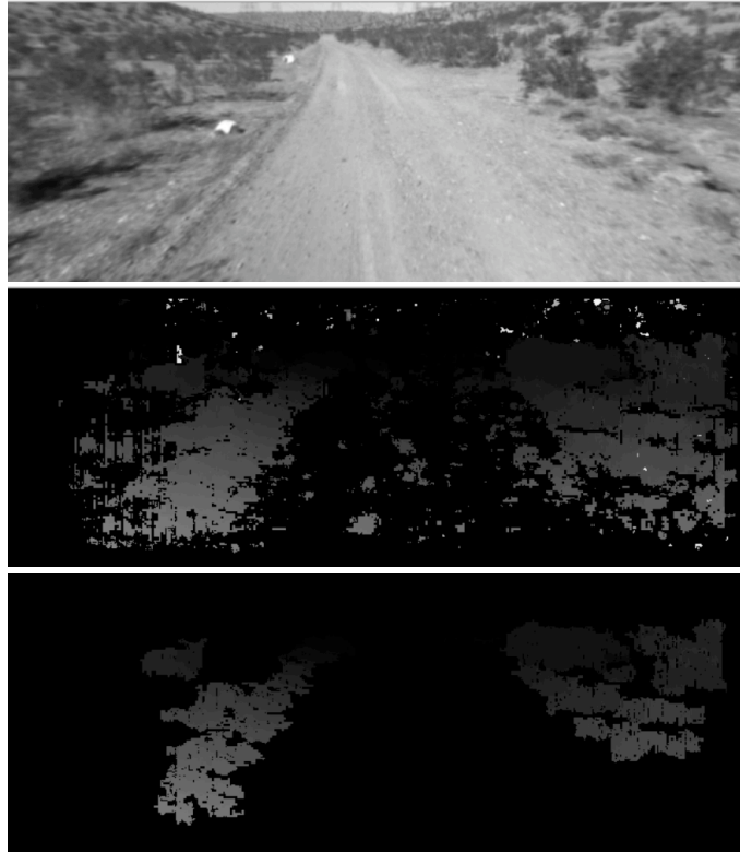
Figure 4: The top image, a typical desert road, is taken by the left long range camera. The middle image is the disparity image before the blob filter is applied – notice the spurious objects in the upper part of the image. The bottom image is the disparity image after the blob filter is applied (minimum region size = 350, connectedness tolerance = 8).
