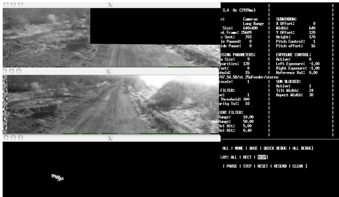
Figure 3. Screenshot when sun covering is active and Alice is facing the sun. On the left side from the top; left image, right image and disparity image. On the right; the display.
