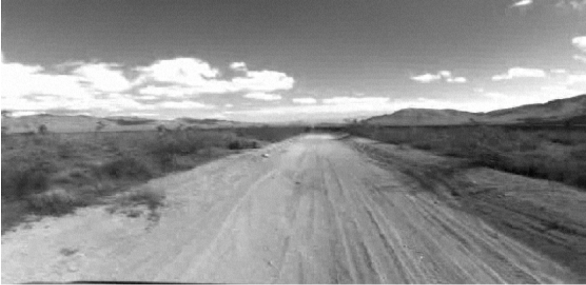
Figure 1a. Whole image when using automatic exposure control and NOT facing the sun.
