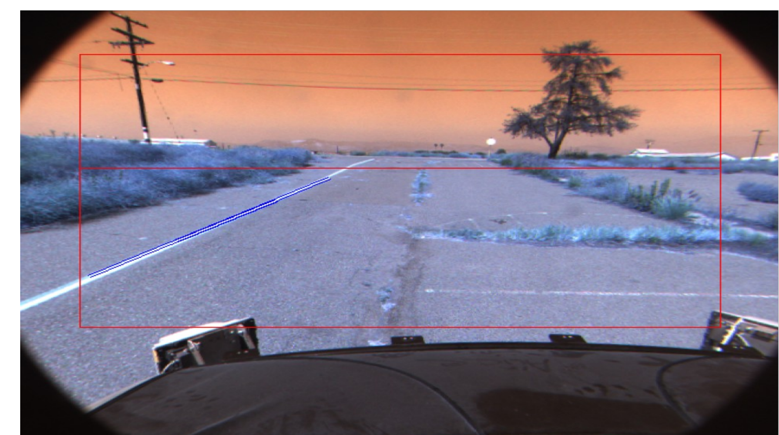
This is what Alice sees with the left camera of the stereo pair. For visualisation, the corrected line gets displayed with its edges painted blue.
