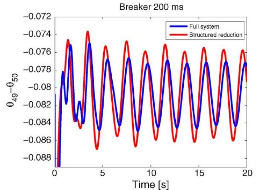
Fig. 13. Responses of  $\theta_{49} - \theta_{50}$  after opening a line for 200 ms.
