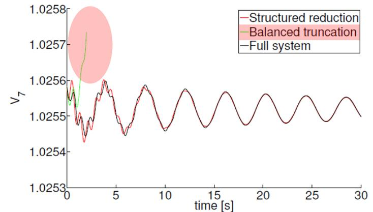
Fig. 5. Transients of  $V_7$  at the tie-line bus with a third order system  $\hat{G}$ .
