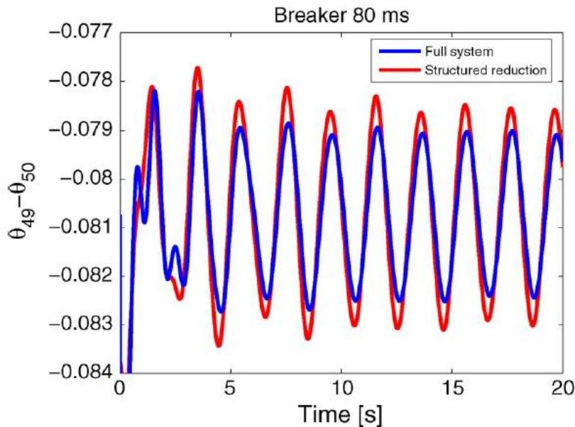
Fig. 12. Responses of  $\theta_{49} - \theta_{50}$  after opening a line for 80 ms.
