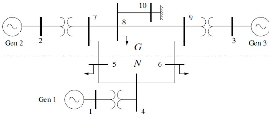
Fig. 3. The WSCC 3-machine, 9-bus system with an infinite bus.
