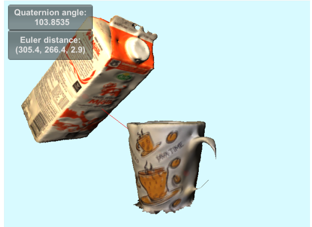
Fig. 5. Example of the rotation feature extracted between a pair of objects. The distance between quaternions measure the distance in all dimensions. The euler distance measures the distance between each dimension separately.
