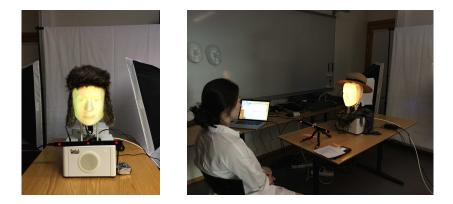
**Fig. 1.** The interactive gaze model is implemented on a talking social robot head Furhat. An eye tracker is placed in front to detect users' gaze.
