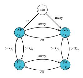
Fig. 2. State transition diagram for our interactive mutual gaze model. *On* denotes when user is detected as looking towards the robot. *Away* denotes when user is averting their gaze from Furhat.
