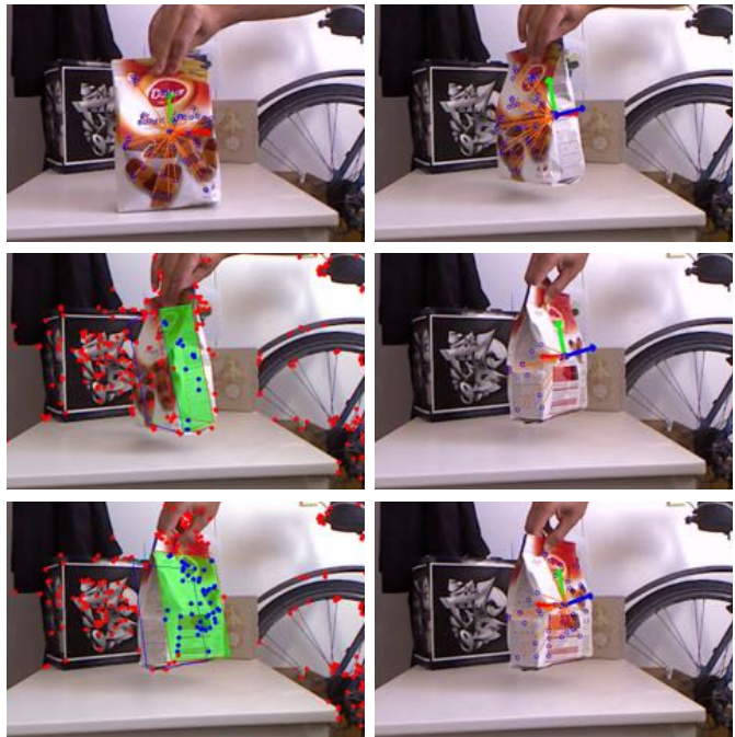
Fig. 1. Tracking and incremental learning. Initially (top left) the method knows only the appearance of the object facing the camera. Its depth is furthermore unknown. Current appearance measurements are used to estimate the pose of the object and together with depth measurements adjust the inscribed cuboid (right). As new sides of the object become visible (mid and bottom left), the cuboid is used to determine which measurements are added to the object model (blue points) and which are discarded (red points).
