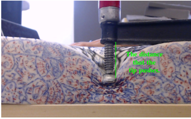
Fig. 7. The flat edge of the clamp’s screw is moved to the same end position for each foam.
