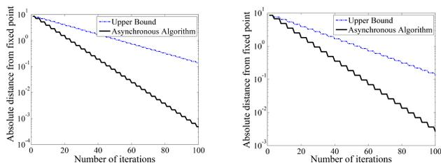
Fig. 2. Upper bound and actual convergence rate of (24) for user 3 (left) and user 4 (right) in the wireless network described in Example 2. The horizontal axis represents the number of iterations and the vertical axis shows  $\frac{1}{v_i} |p_i(t) - p_i^*|$ ,  $i = 3, 4$  (in logarithmic scale).
