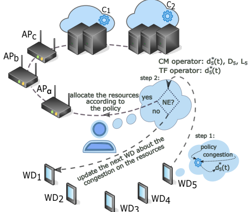
Fig. 4. Example of the information exchange between the operator and WD 1 and WD 5 .
