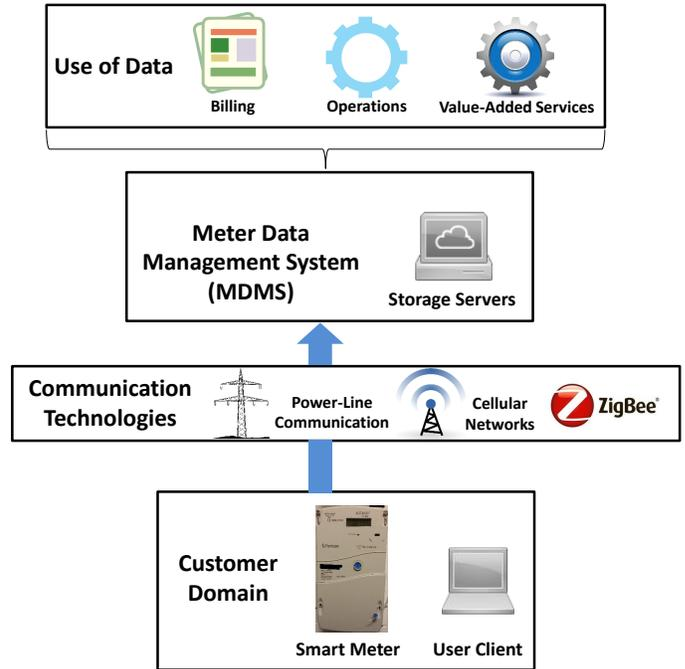
Fig. 1. Different domains of the smart metering infrastructure.
