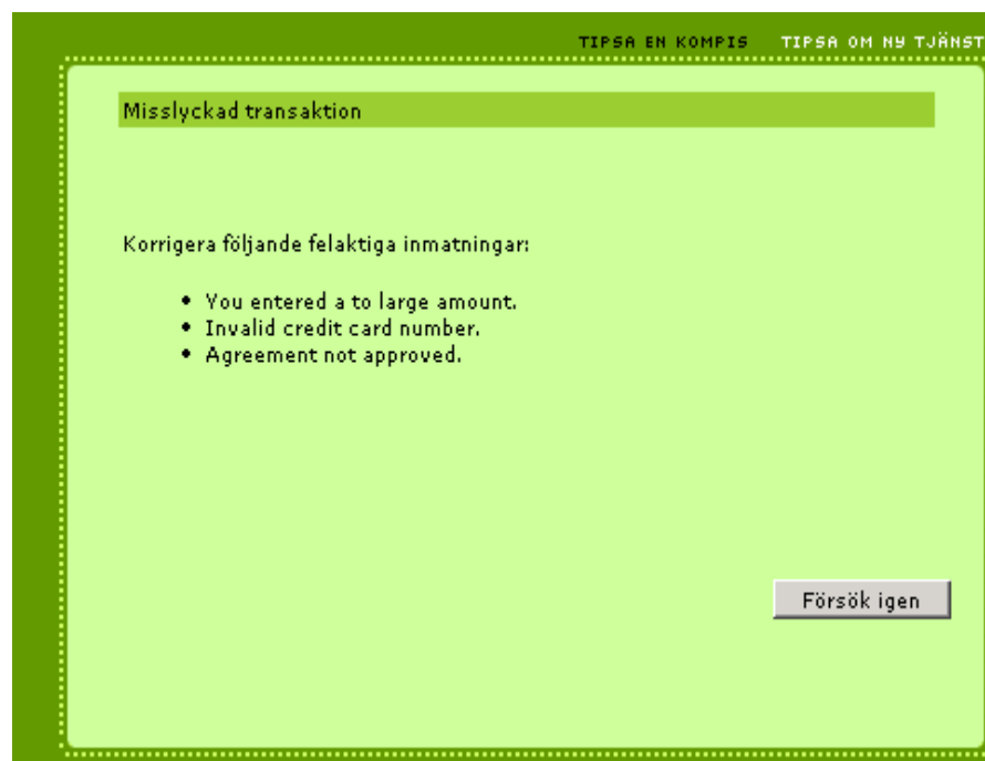
Figure 12.6. Failure page. This page is displayed when everything is not ok. In this example the user has entered a too large amount, an invalid credit card number and has not checked the agreement checkbox.
