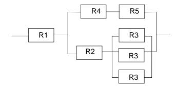
$$R_{system} = R_1(1 - (1 - R_4 R_5)(1 - R_2(1 - (1 - R_3)^3)))$$
