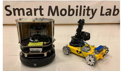
Fig. 1: TurtleBots (left) and Nexus 4WD Mecanum Robotic Cars (right) are used in the experiments in Section IV.
