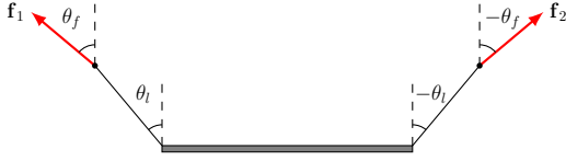
Fig. 3: Definition of the angles \theta_f and \theta_l . The system is assumed symmetric with respect to the center of the bar. The variable \theta_l corresponds to the angle between the cable and inertial Z-axis, while \theta_f corresponds to the angle between the thrust F_i being applied on the cable and the inertial Z-axis.
