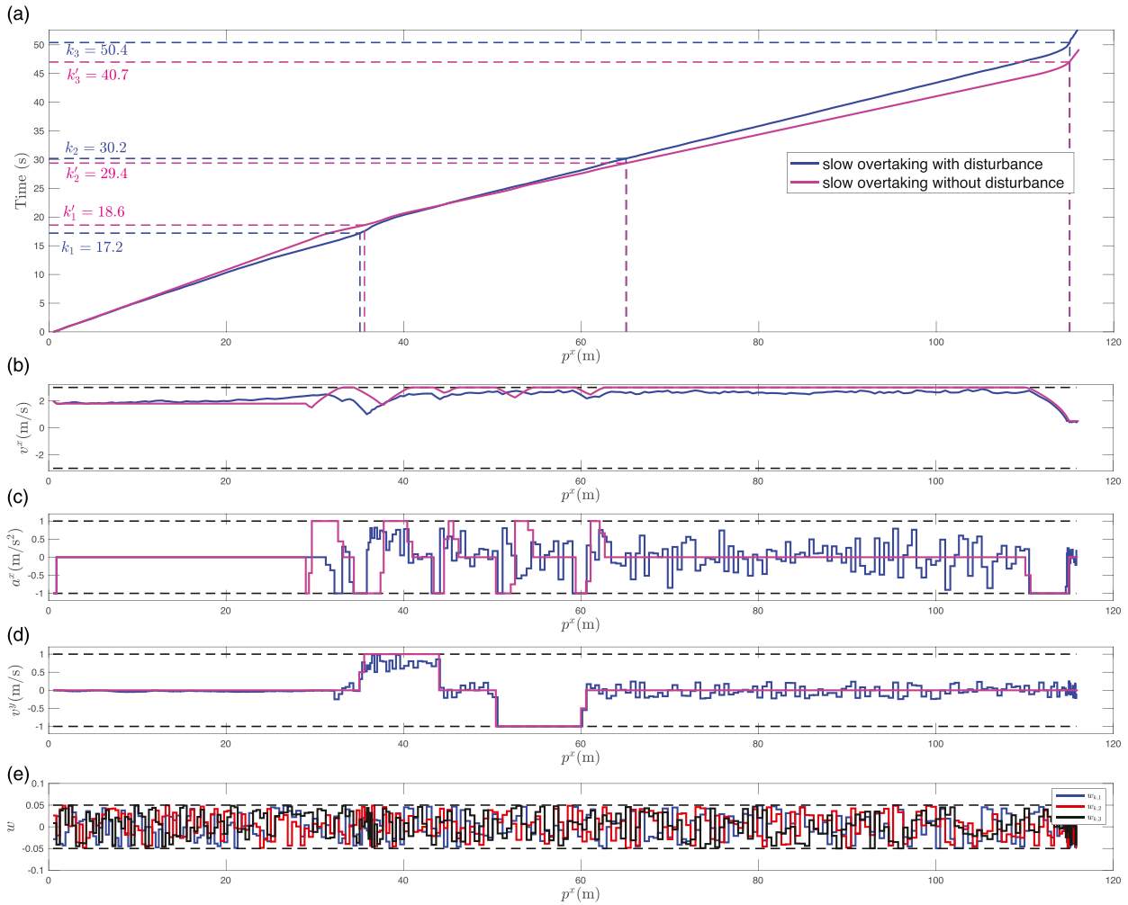
Figure 15. Comparison of robust control with noise and deterministic control without disturbance signal in the ast overtaking in the slow overtaking: (a) position-time trajectory; (b) velocity trajectory of x-axis; (c) control trajectory of x-axis; (d) control trajectory of y-axis; (e) disturbance signals.
