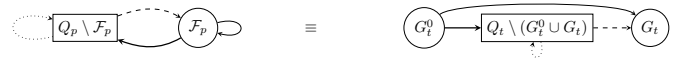
Fig. 1: Construction of \mathcal{A}_t (right) from \mathcal{A}_p (left). Similar node shape (resp. line style) represents equivalent state sets (resp. transition function between sets).
