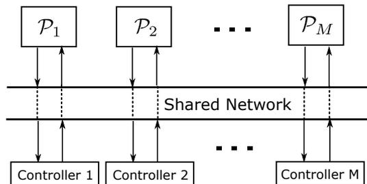
Fig. 1. Networked Control System considered in this paper. Each plant  $\mathcal{P}_i$  ( $i \in \mathcal{M}$ ) is controlled by the corresponding controller  $i$  through a shared network.
