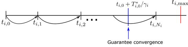
Fig. 4. The cost function is given by (15) such that  $t_{i,k}$  approaches  $t_{i,max}$  as soon as possible. Due to the constraint (16),  $t_{i,N_i}$  is guaranteed to be placed between  $t_{i,0} + T_{i,0}^*/\gamma_i$  and  $t_{i,max}$ .
