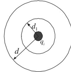
Fig. 1. Each agent has sensing radius  $d$ . For the collision avoidance objective, it requires knowledge of the positions of agents at distance less than  $d_1 < d$  at each time instant.
