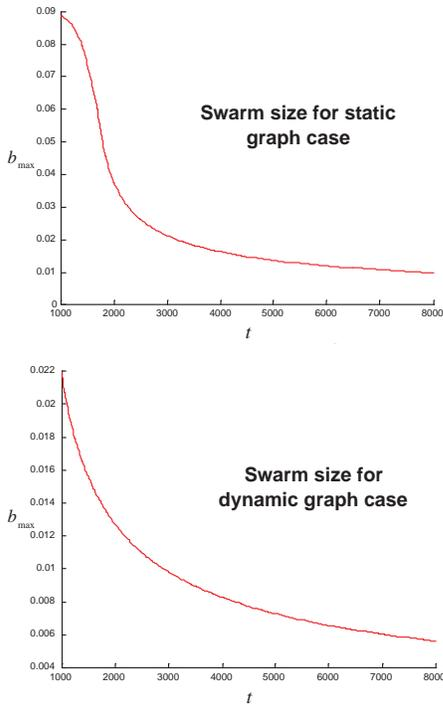
Fig. 3. Evolution of the swarm size for the two simulations of Figure 2. The dynamic graph formulation leads to a smaller swarm size.
