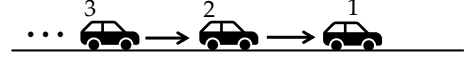
Fig. 2. Simulation scenario. Each vehicle is able to measure relative state information with respect to the vehicle in front using on-board sensors (indicated as solid arrows).
