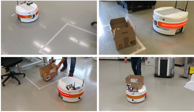
Fig. 12. Example situations during Experiment I. Shown top are cases when the robot did not (left) or did (right) observe a product for delivery. Shown bottom is the transportation process.
