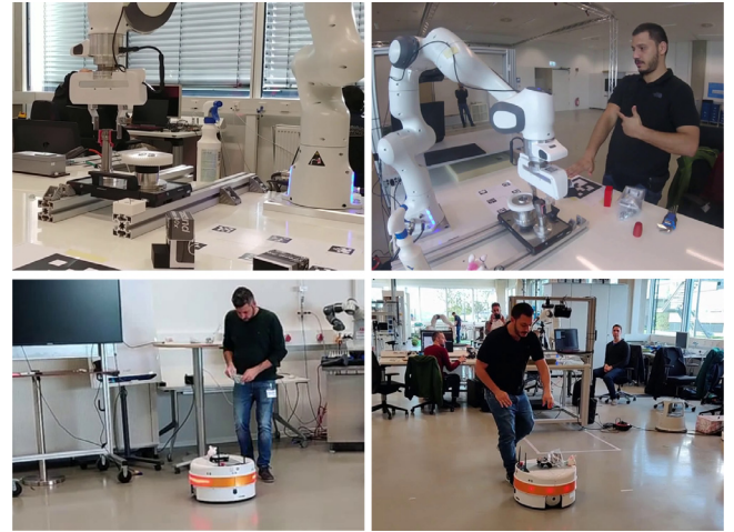
Fig. 13. Example situations during Experiment II. The assembly station follows an assembly routine (top left) and the human worker requests supplies when needed (top right). Shown bottom is the delivery of requested supplies.
