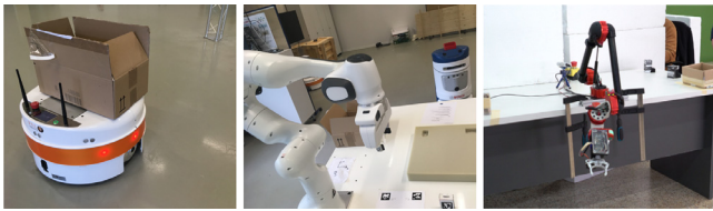
Fig. 10. Different types of robots used in the experiments. From left to right: (1) TIAGo Base by PAL Robotics, (2) Panda by Franka Emika, (3) A-2085-06 by Hebi Robotics.
