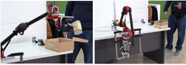
Fig. 14. Example situations during Experiment III. The assembly station is explicitly modeled by a pick-and-place routine (left) and only when done, the human worker may request supplies (right).
