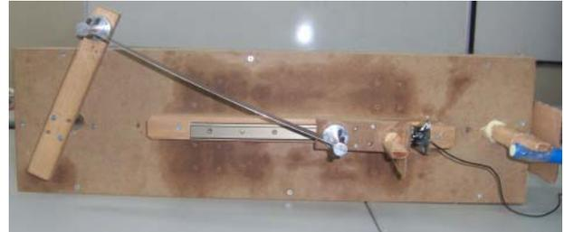
**Fig. 9:** The rigid mode of the slider crank mechanism
