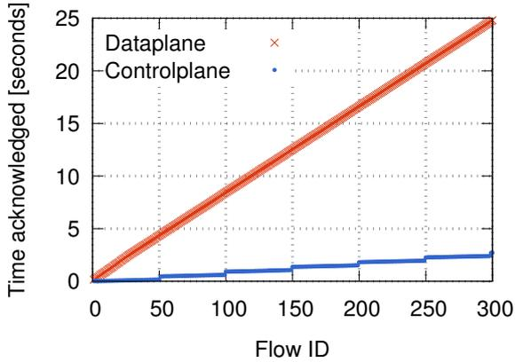
Figure 5: Control plane confirmation times fall behind the data plane probe results in HP 5406zl when using rules with different priorities. The scale of divergence is unlimited.
