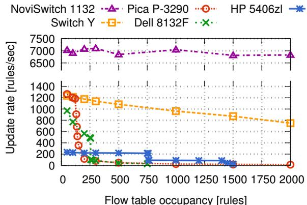
Figure 13: Priorities cripple performance — Experiment from Figure 12 repeated with a single additional low-priority rule installed reveals a massive fall in performance for two of the tested switches.
