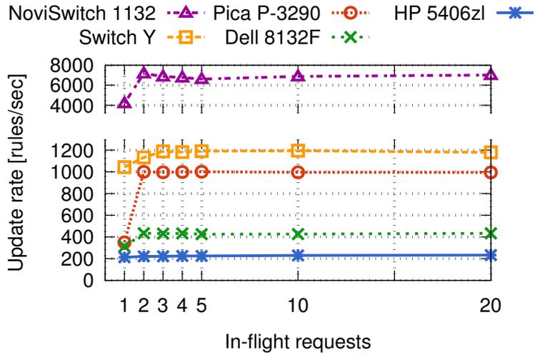
Figure 10: Switch performance increases with the number of in-flight requests. However, the improvements beyond the case where the controller waits for confirmation of the previous request before sending the next one ( $k = 1$ ) are negligible.
