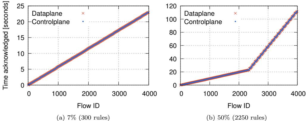
Figure 9: Control plane confirmation times and data plane probe results for the same flows in Switch X (firmware version V2). Data and control plane views are synchronized, but the rate still slows down after about 4600 flow installations.
