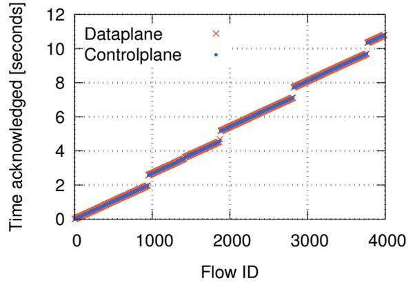
Figure 8: Control plane confirmation times and data plane probe results in Switch Y with 95% table occupancy are synchronized, but the switch stops processing new updates for 600 ms after every 2s.
