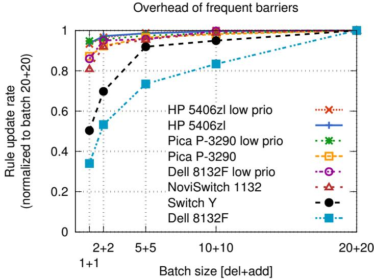
Figure 16: Cost of frequent barriers is modest except for the case of Dell 8132F with no priorities (*i.e.*, with high baseline speed) and Switch Y where the cost is significant.
