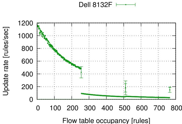
Figure 17: An update rate in Dell 8132F suddenly increases for 4 specific flow table occupancy values.
