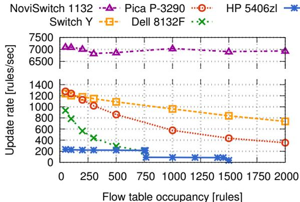
Figure 12: For most switches the performance decreases when the number of rules in the flow table is higher.
