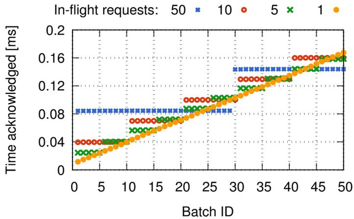
Figure 11: HP 5406zl barrier reply arrival times. HP 5406zl postpones sending barrier replies until there are no more pending requests or there are 29 pending responses.
