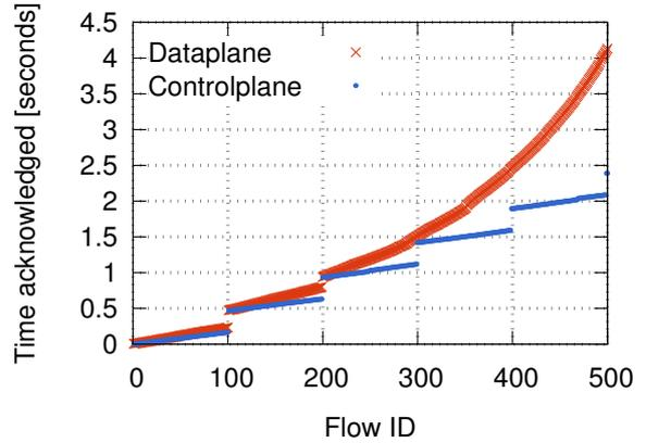
Figure 6: Control plane confirmation times fall behind the data plane probe results in HP 5406zl when filling the flow table.
