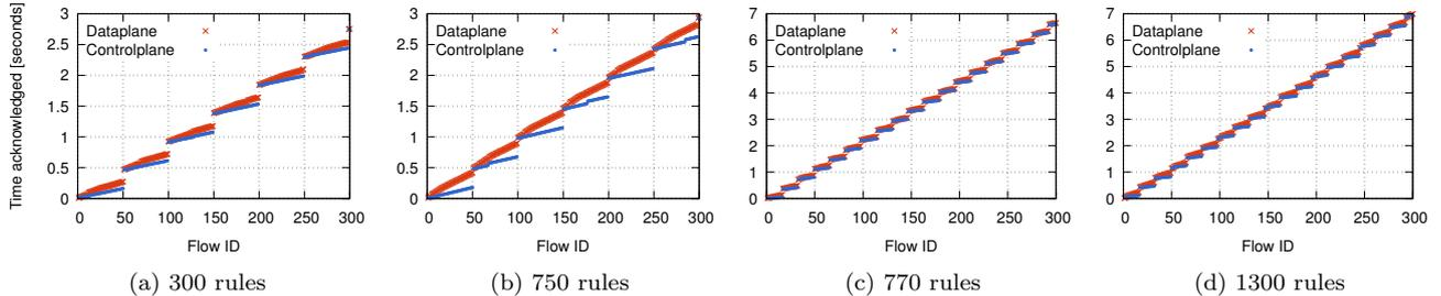
Figure 4: Control plane confirmation times and data plane probe results for the same flows in HP 5406zl depending on flow table occupancy. The rate slows down and the pattern changes for over 760 rules in the flow table.
