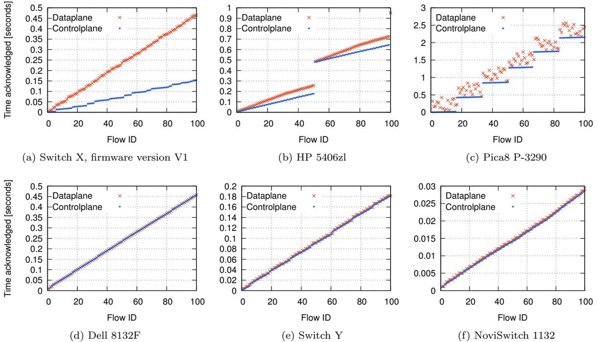
Figure 2: Control plane confirmation times and data plane probe results for the same flows. Switch data plane installation time may fall behind the control plane acknowledgments and may be even reordered.
