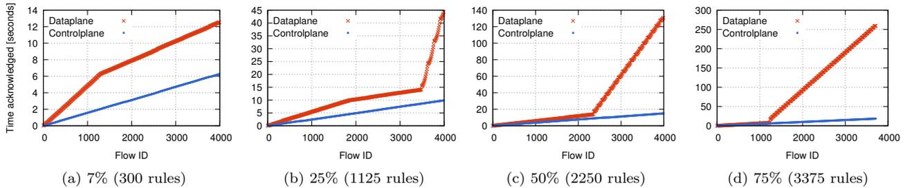
Figure 3: Control plane confirmation times and data plane probe results for the same flows in Switch X (firmware version V1) depending on flow table occupancy. The rate suddenly slows down after about 4600 flow installations (including initial rules installed before the experiment starts).
