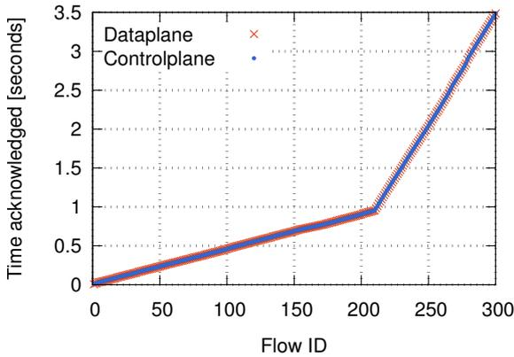
Figure 7: Control plane confirmation times and data plane probe results in Dell 8132F are synchronized, but the update rate suddenly slows down after about 210 newly installed rules.
