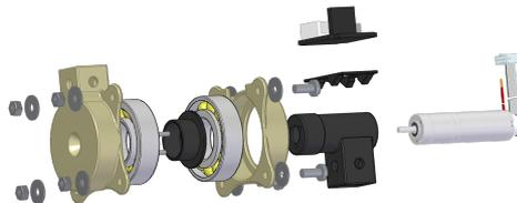
Figure 4: Exploded view of a joint to visualize the construction process.
