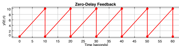
(b) Output of the integrator, using an extrapolating ZCD.
