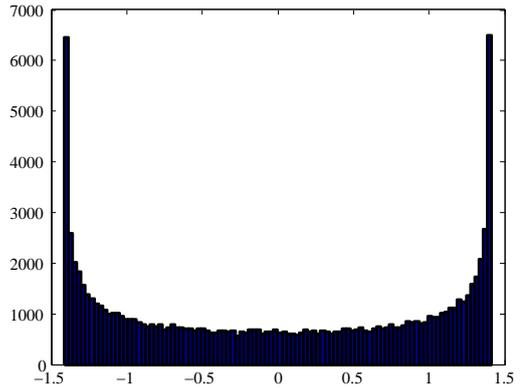
Fig. 3. Histogram of 100000 samples of a pseudo white noise signal generated by the proposed algorithm.
