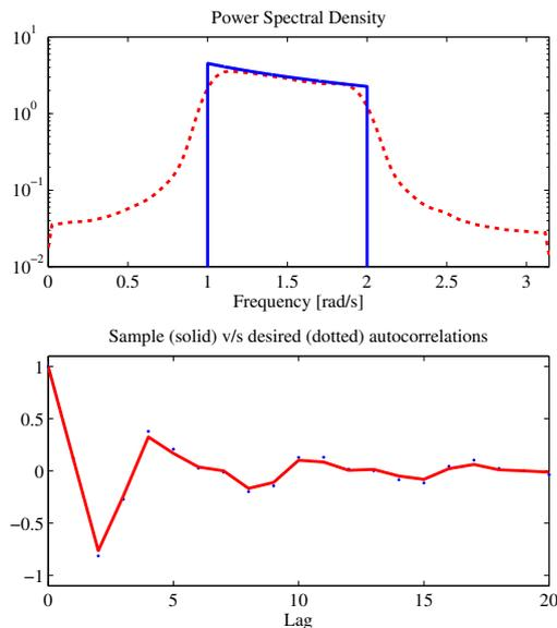
Fig. 5. Sample spectral density (red dotted line) and autocorrelation function of a bandlimited ‘ $1/f$ ’ noise signal generated by the proposed algorithm. The ideal bandlimited ‘ $1/f$ ’ noise spectrum for  $\underline{\omega} = 1$  and  $\bar{\omega} = 2$  is also shown (solid blue line).
