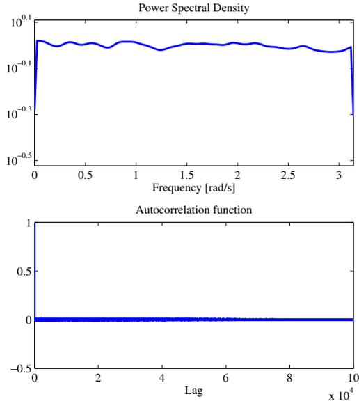
Fig. 1. Sample spectral density and autocorrelation function of a pseudo white noise signal generated by the proposed algorithm.
