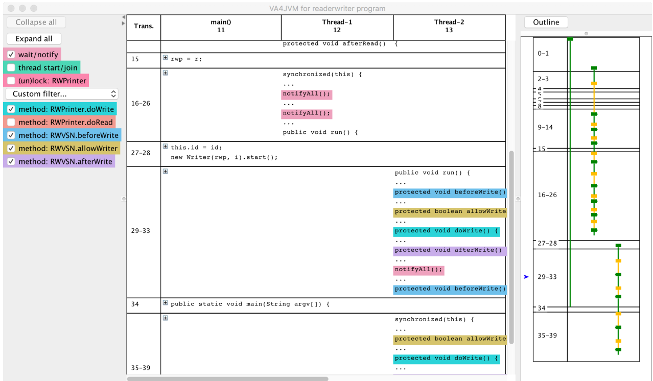
Fig. 3. Screenshot of VA4JVM, for analyzing a reader-writer example with one reader and one writer thread. The left panel shows the filters, the central panel part of the execution (zoomed out), and the right panel shows the thread state view. In the thread state view, the yellow (green) bars represent locking (unlocking) operations; a vertical line shows the lifetime of a thread while holding a lock (in yellow) or no lock (in green).
