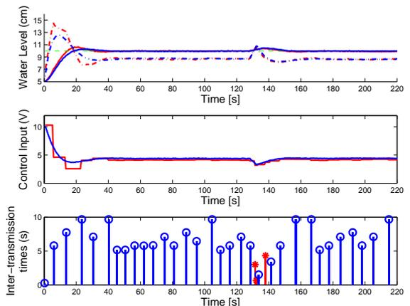
Fig. 7: Experimental results for hybrid communication. Signal legends are shown as in Fig. 5. The red star marker represents an event-based transmission and the blue round marker represents a predictive transmission.
