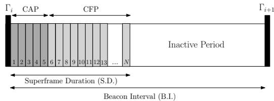
Fig. 3: Superframe structure of the modified IEEE 802.15.4 MAC.
