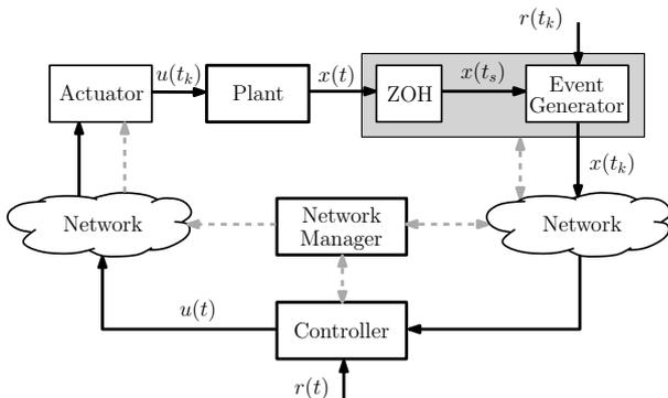
Fig. 2: System architecture for an aperiodic networked control loop.
