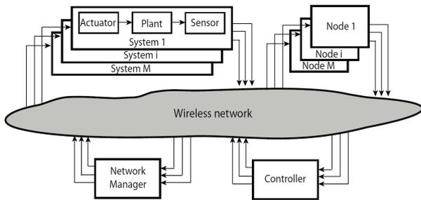
Fig. 1: Wireless networked control system.
