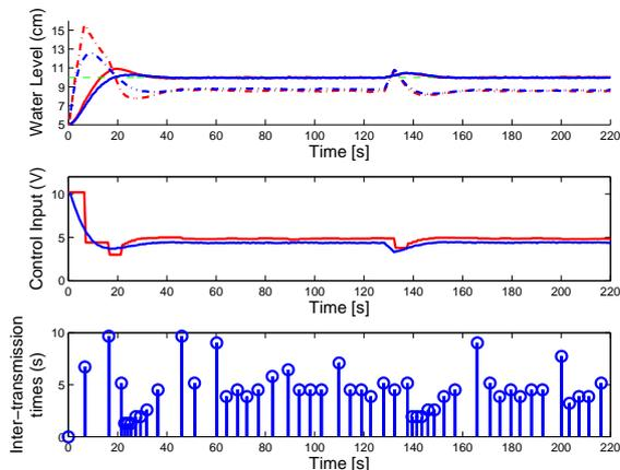
Fig. 5: Experimental results for event-based communication. The upper plot depicts the evolution of the water tank level and middle plot the control input values for event-based mechanism (red) and a periodic controller (blue). Upper (dash-dotted line) and lower (solid line) water levels are presented.
