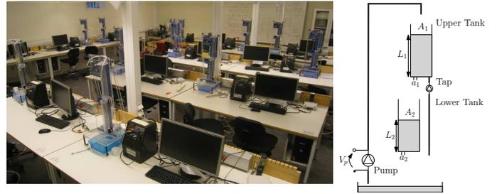
Fig. 3: Double-tank system testbed at KTH Royal Institute of Technology and the diagram of a double-tank system.
