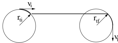
Figure 4.7: The parallelity of the tangent vector, is not a sufficient condition for path feasibility. The thicker line clearly is not a continuously differentiable path.
