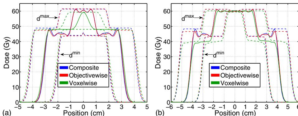
FIG. 11. (a) Worst case dose distributions associated with the plans depicted in Fig. 2(b). (b) Corresponding worst case doses with respect to a 6 cm wide target.
