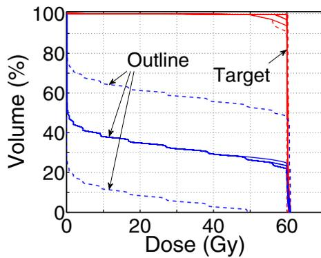
FIG. 12. DVHs for the worst case dose distributions  $d^{\min}$  and  $d^{\max}$  associated with the plan depicted in Fig. 2(b) (dashed). DVHs for the scenario dose distributions are shown for reference (solid). The outline is the union of the rectum and bladder.
