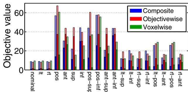
FIG. 7. Objective value in various scenarios for the optimal dose to the symmetric formulation for the 3D geometry (lt=left, rt=right, pos=posterior, ant=anterior, sup=superior, inf=inferior). The dark-colored parts of the bars indicate target constituent's contribution to the total objective value.
