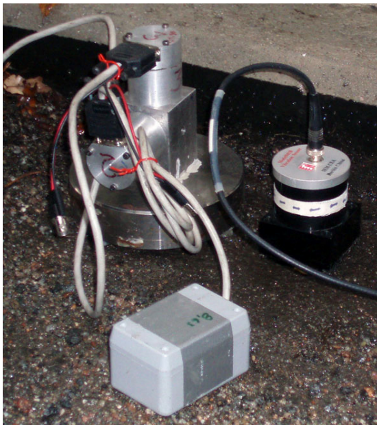
Figure 3.1: Assembly of accelerometers, MEMS accelerometer on the left mounted to a heavy steel weight, Ultra-Low Frequency Gauge on the right. The lower gray box is a power supply consisting of one 9V battery.
