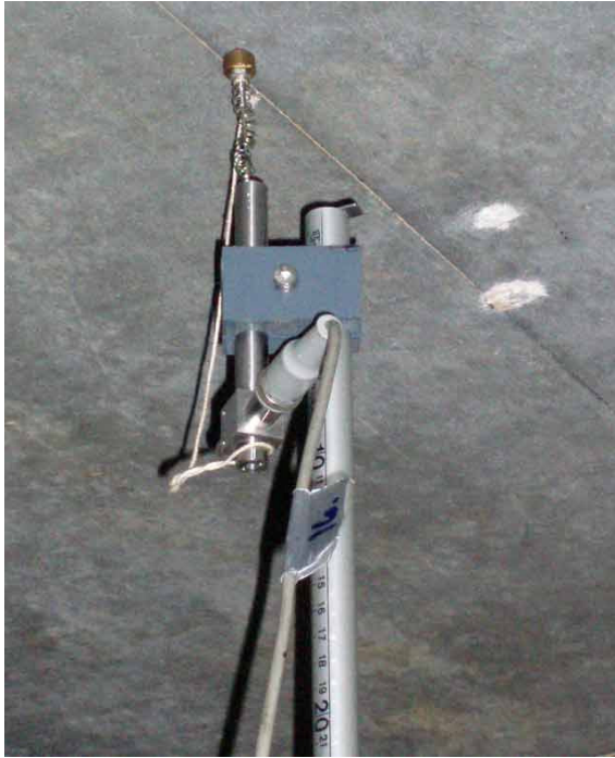
Figure 3.2: Position of the LVDT in contact with the bottom of the bridge deck.
