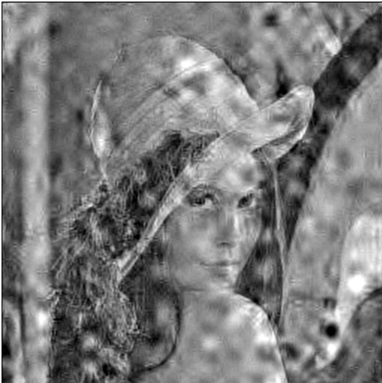
Figure 5.3. Result from subband coder using regular VQ at 0.5 bits/pixel, designed assuming no channel errors, when subject to 10% bit-losses and 5% bit-errors in the actual channel.
