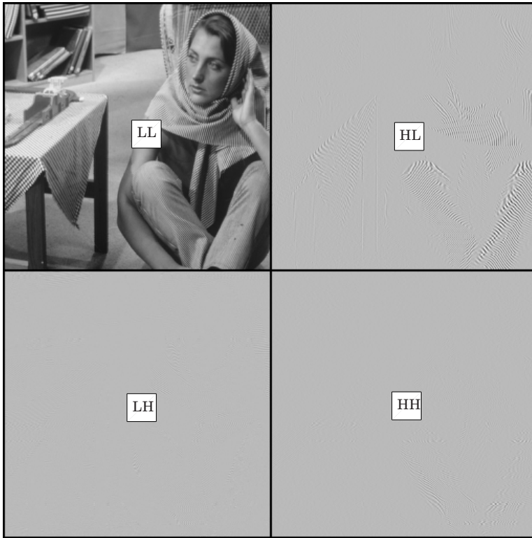
Figure 4.5. Illustration of the effects of a subband transform on the Barbara image. Subbands are placed next to each other to keep the original dimensions with lowest frequency to the top left.
