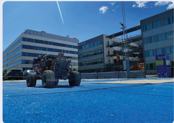
FIGURE S5 The KTH Smart Mobility Lab SVEA platform integrated into the Kista Innovation Park, where a private 5G network is deployed to support small-scale connected vehicle experiments.
