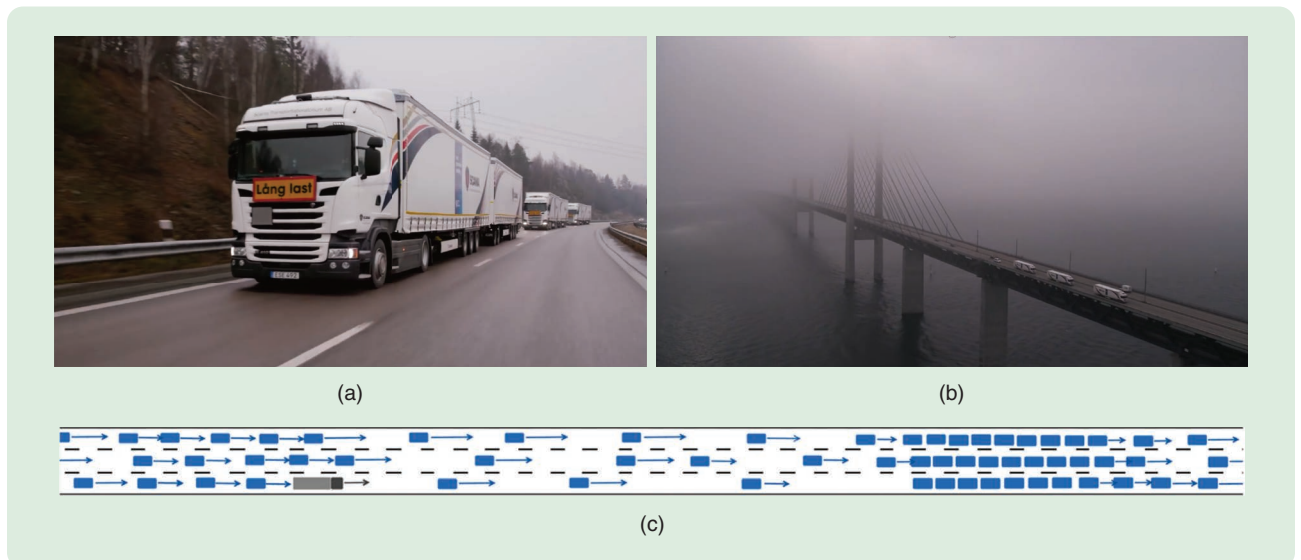
FIGURE 10. When (a) a three-vehicle truck platoon drives on (b) a highway, it acts as (c) a moving bottleneck with respect to the rest of the traffic. (Source: Scania; used with permission.)
