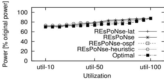
Figure 6: Power consumption for different traffic demands in the Genuity topology.
