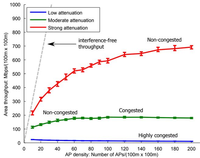
Fig. 5. Area throughput for single channel deployment, 10 to 200 WLANs. Same parameters as fig. 4.
