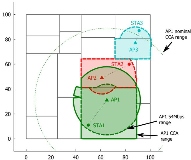
Fig. 2. Example network topology highlighting hidden node and exposed node situations.
