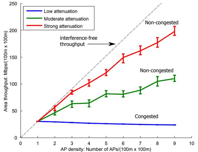
Fig. 4. Area throughput for single channel deployment, 1 to 9 WLANs. Low attenuation: No walls,  $\alpha = 2$ ,  $P_t = 100$  mW. Moderate attenuation: Moderate wall density,  $\alpha = 3$ ,  $P_t = 100$  mW. Strong attenuation: High wall density,  $\alpha = 3$ ,  $P_t = 100$  mW.
