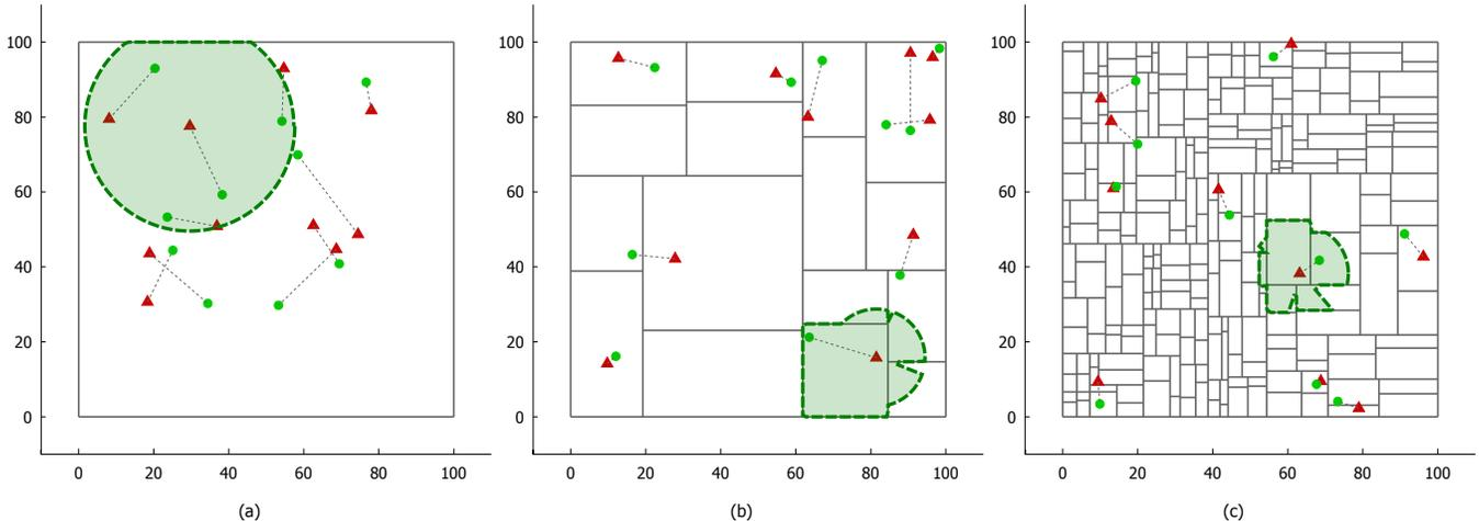
Fig. 1. Example network topologies and floor plans containing 10 links. AP–STA pairs are represented by a connected triangle and circle. For all figures, transmit power is 100 mW, pathloss exponent is 3, the 54 Mbps coverage range of an example AP is highlighted. (a) Open area. (b) Moderate wall density: 16 rooms. (c) High wall density: 256 rooms.
