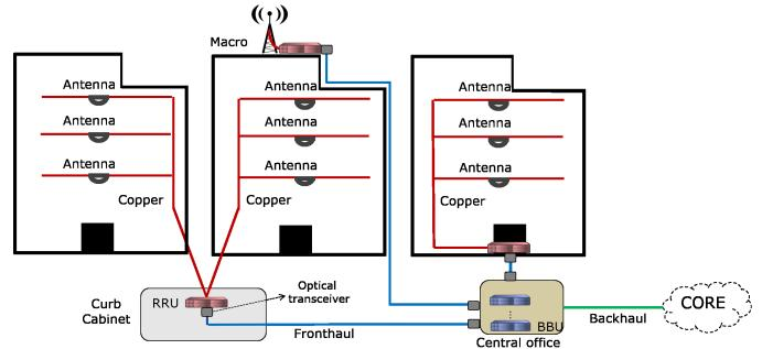
Fig. 1. The Centralized Radio Architecture (CRA) concept.
