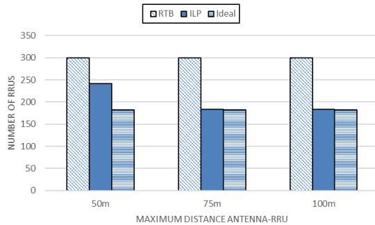
Fig. 3. Number of RRUs as a function of the maximum distance between antenna and RRU.
