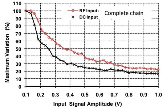
Figure 4. Maximum variations in RF responses before calibration.
