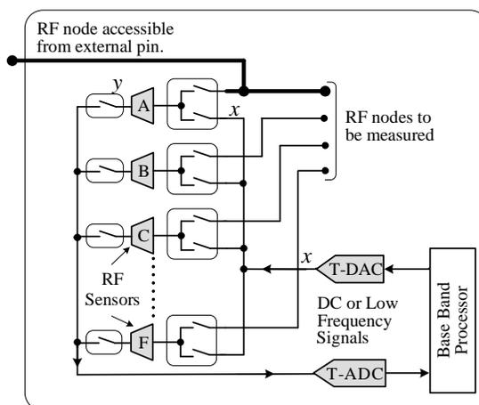
Figure 1. Architecture of calibration circuitry.
