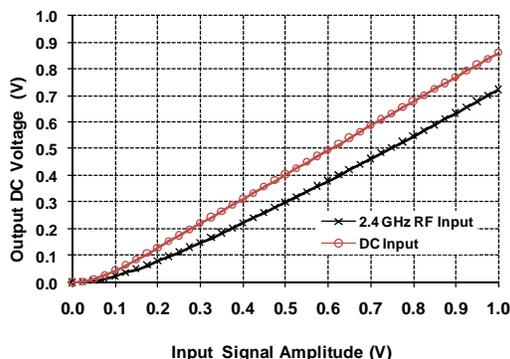
Figure 2. Typical ch-cs of RF sensors designed in 65 nm CMOS.
