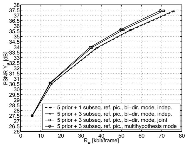
Figure 4: PSNR of the B picture luminance signal vs. B picture bit-rate for the CIF sequence *Flowergarden* with 30 fps. Two B pictures are inserted after each inter picture.  $QP_B = QP_P$ . The multihypothesis mode is compared to the bi-directional mode.
