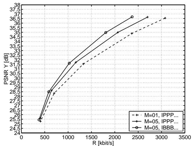
Figure 7: PSNR of the luminance signal vs. overall bit-rate for the CIF sequence *Mobile & Calendar* with 30 fps. Generalized B pictures with forward-only prediction are compared to inter pictures.
