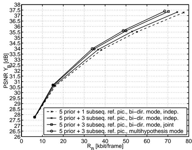
Figure 3: PSNR of the B picture luminance signal vs. B picture bit-rate for the CIF sequence *Mobile & Calendar* with 30 fps. Two B pictures are inserted after each inter picture.  $QP_B = QP_P$ . The multihypothesis mode is compared to the bi-directional mode.
