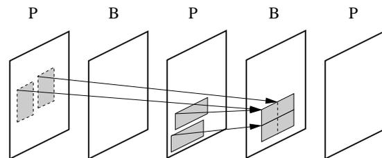
Figure 2: The multihypothesis mode also allows a linear combination of two past macroblock prediction signals.
