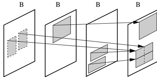
Figure 5: Generalized B pictures with forward-only prediction utilize multiple reference picture prediction and multihypothesis motion-compensated prediction. The multihypothesis mode uses two hypotheses chosen from past reference pictures.
