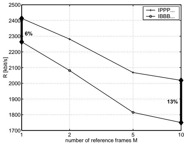
Figure 6: Average bit-rate at 35 dB PSNR vs. number of reference pictures for the CIF sequence *Mobile & Calendar* with 30 fps. Generalized B pictures with forward-only prediction are compared to inter pictures.
