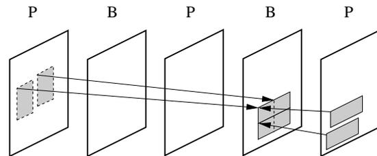
Figure 1: A bi-directional prediction mode allows a linear combination of one past and one subsequent macroblock prediction signal. The inter pictures are denoted by P.
